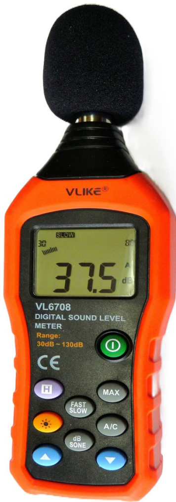
Fig. 1. VLIKE Model VL6708 digital sound meter.
